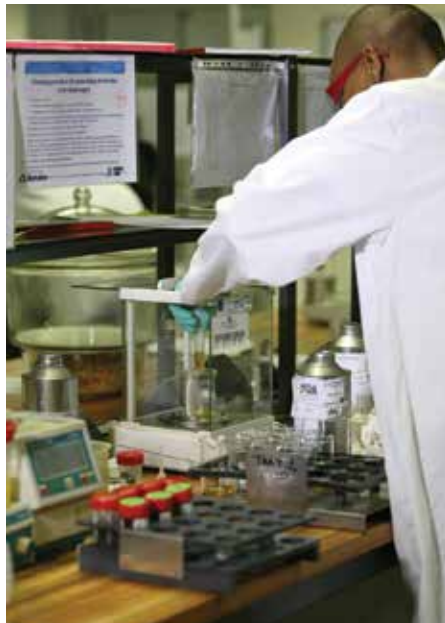
A WearCheck laboratory technician processes used oil samples to test for trace elements of contamination - information which provides important clues about a machine's condition.
